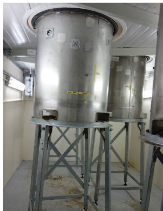
Figure 1. The New Zealand Biotron, controlled environment growth chamber above and independently controlled rhizotron below.
