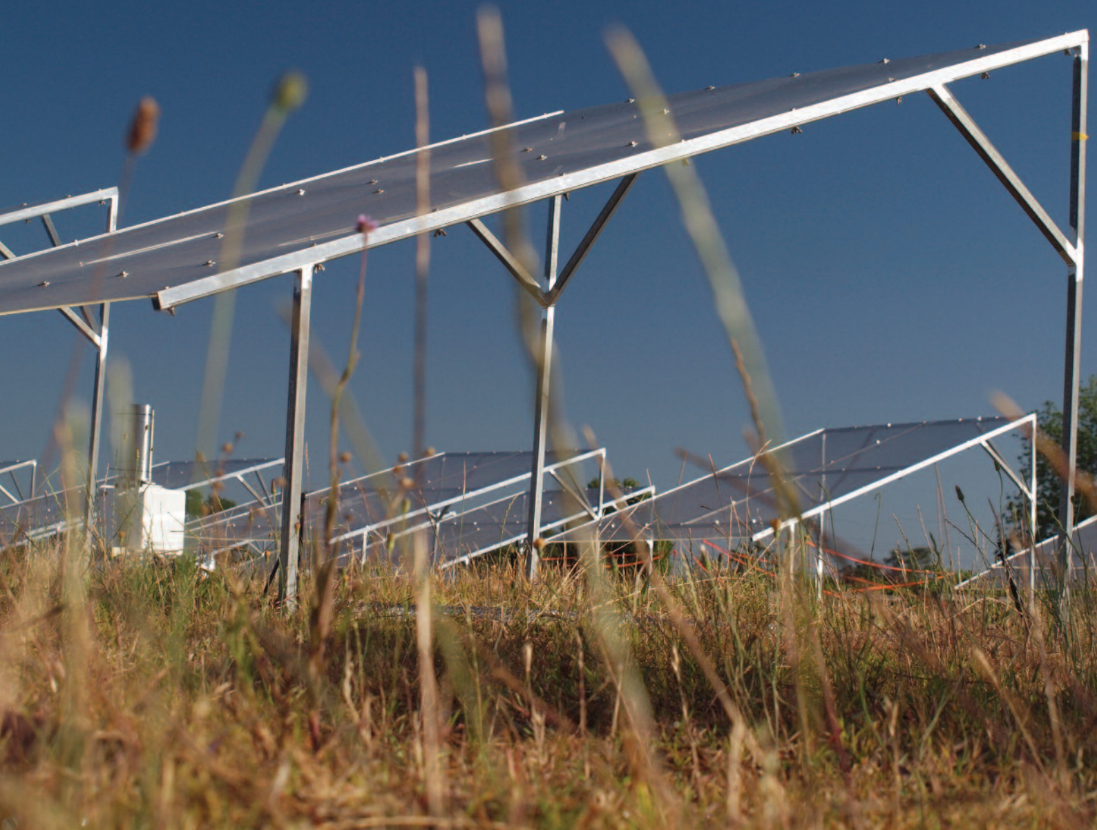
Figure 6. The rain shelters of the new DRI-GRASS facility.
